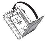
**4** Remove the black film cover that is automatically ejected from the camera.
