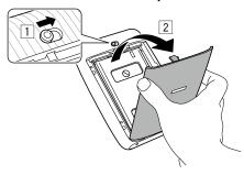
**2** Grasp the rectangular holes on the film pack, then pull film pack out from the printer.
