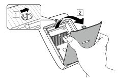
2 Insert film pack by aligning the yellow marks.
