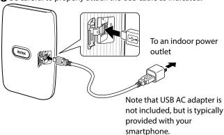
Connect the printer with a USB AC adapter supplied with your smartphone (not included with INSTAX Mini Link printer) using the supplied USB cable, then connect the USB AC adapter to an indoor power outlet.
