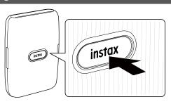
Press and hold the Power button for approximately 1 second to turn the printer on or off.
