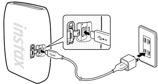
Connect the printer with a USB AC adapter (sold separately) using the supplied USB Type C cable, then connect the USB AC adapter to an indoor power outlet. A USB AC adapter is not included with the INSTAX MINI LINK 3 Smartphone printer (though it may have been supplied with your Smartphone).
