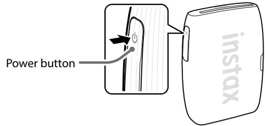
Press and hold the Power button for approximately 1 second to turn the printer on or off.
