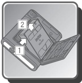
How to remove the INSTAX SQUARE instant film cartridge once all film sheets have been used.
